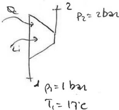
$Q_e + L_i = \Delta i = c_p (T_2 - T_1)$
